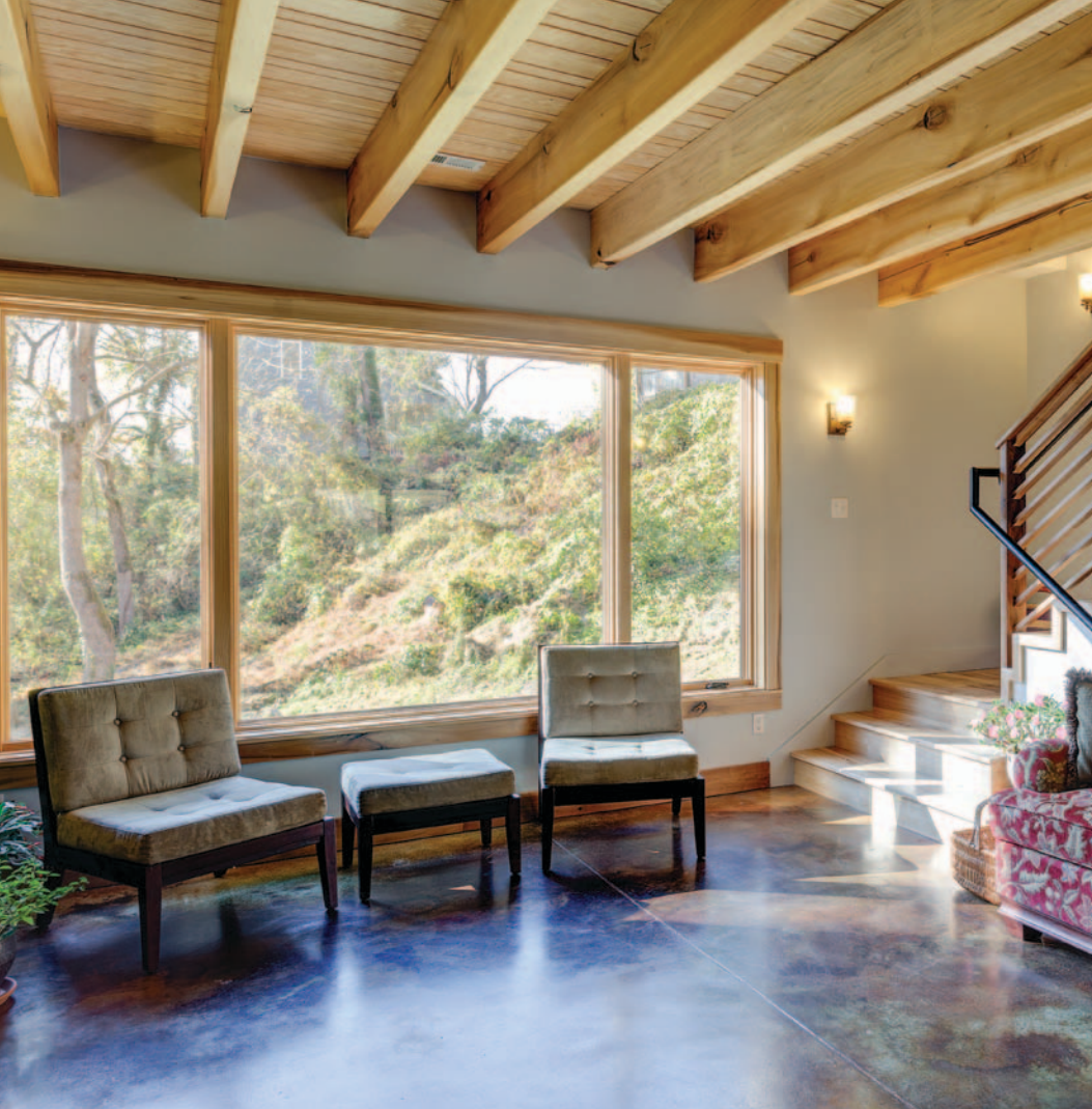
Sunny side up. Extensive glazing on the south side of the house captures winter sun on the bleakest days, and the thermal mass of the concrete floor harnesses it.
